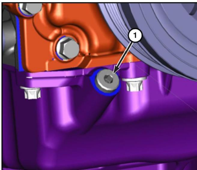
2. Insert the [Dipstick 2025600210](#) (1) into the oil level check port until seated squarely on the port opening. Remove the tool and note the oil level (2).
