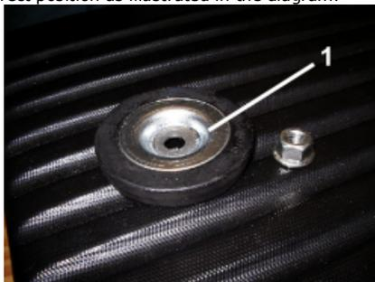
1. If the plate is not fitted in the correct position, refit it correctly as illustrated in the diagram.
